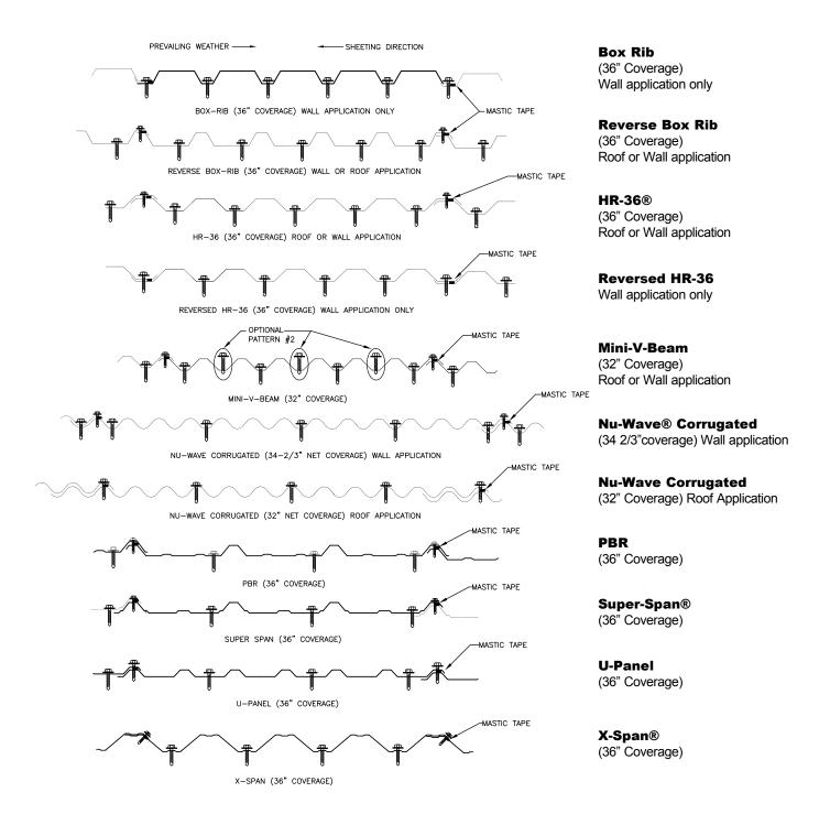
**Note:** Lap panels away from prevailing weather. Use only those accessories specifically designed for use with this product. Use only galvanized or Zincalume®-coated fasteners. Isolate roofing and flashings from contact with dissimilar metals. Fastener selection will vary based upon substrate. The use of butyl mastic tape along the sidelaps, as shown above, is always recommended for roof panels. Space lap screws @ 18" o.c. maximum.
